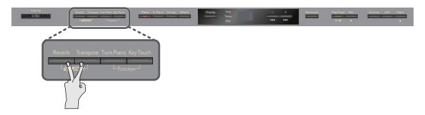
Hold down the [Reverb] button and press the [Transpose] button.
